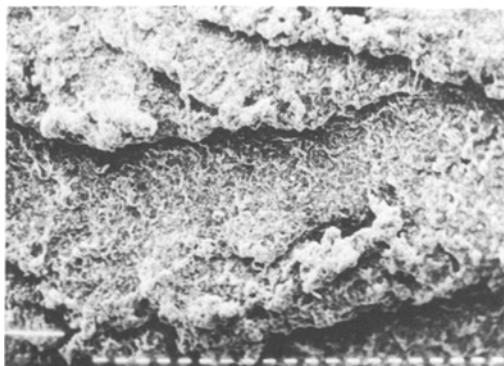
Figure 4 Coarse abrasion pattern (Akron abrader, mix A, \times 21 ).
