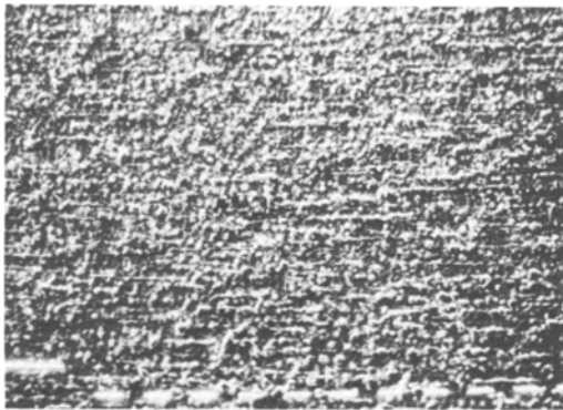
Figure 19 Scratch marks on the surface (Du Pont abrader, mix B, \times 42 ).
