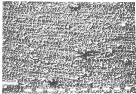
Figure 22 Abrasion pattern in the early stages of formation (Du Pont abrader, mix D, \times 42 ).
