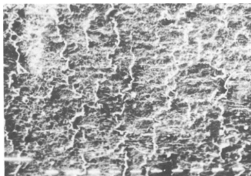
Figure 17 Ridges running perpendicular to the direction of abrasion (Du Pont abrader, mix A, \times 42 ).
