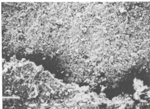
Figure 15 Coarse ridges (DIN abrader, mix C, \times 42 ).
