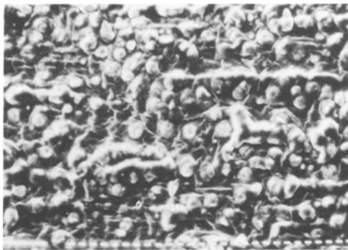
Figure 20 Ball formation on the surface (Du Pont abrader, mix B, \times 170 ).
